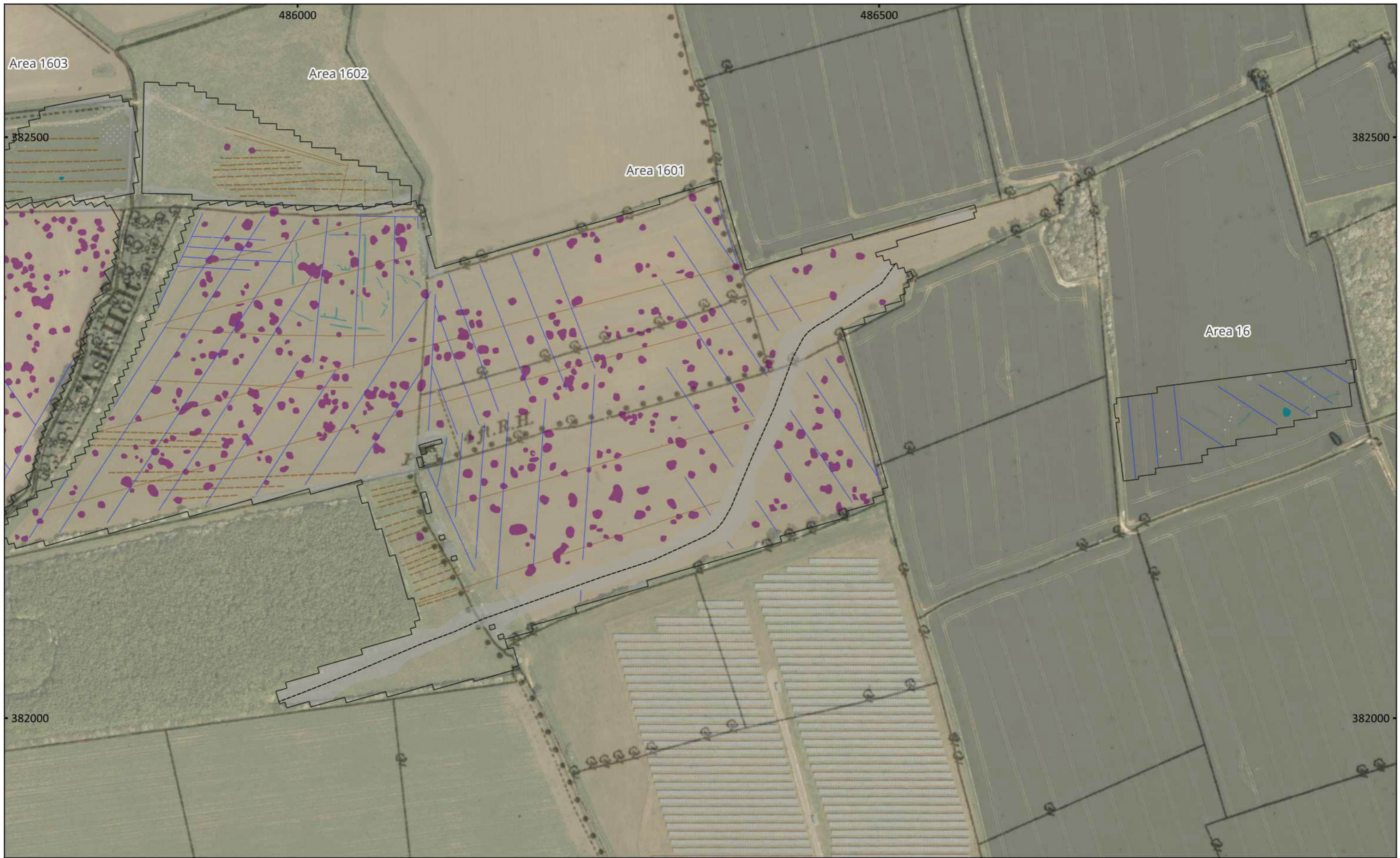
MSSK1393C - Tillbridge Solar Scheme, Cable Route, Willingham-by-Stow, Lincolnshire Figure 10 - Magnetic Interpretation Over Historical Maps and Satellite Imagery (Overview) (Areas 16, 1601 & 1602) 1:3,000 @ A3 Copyright Magnitude Surveys Ltd 2023 Contains historical mapping © CLS Data 2023: Ordnance Survey, 6" 2nd edition c. 1882-1913 Contains Satellite Imagery © Bing 2023
